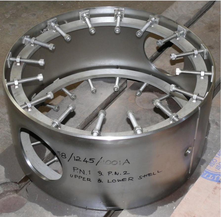
Cylindrical Shell with Fixture before Weldment
