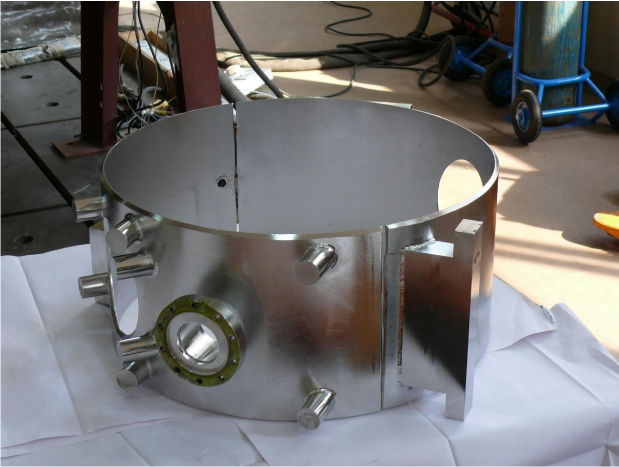
Shell after weldment and electro polishing at CDM, BARC
