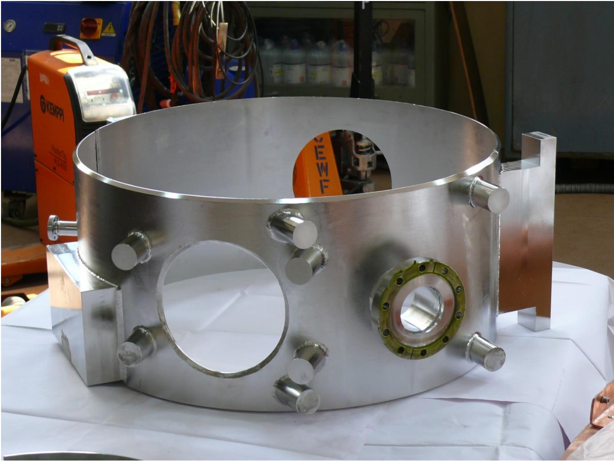
Shell after weldment and electro polishing at CDM, BARC
